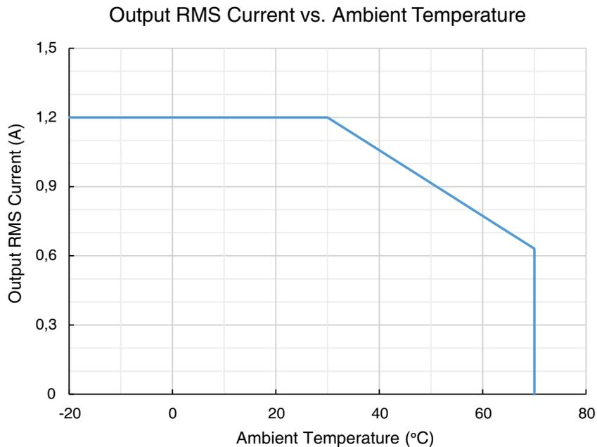
Picture 4. Output RMS Current vs. Ambient Temperature
